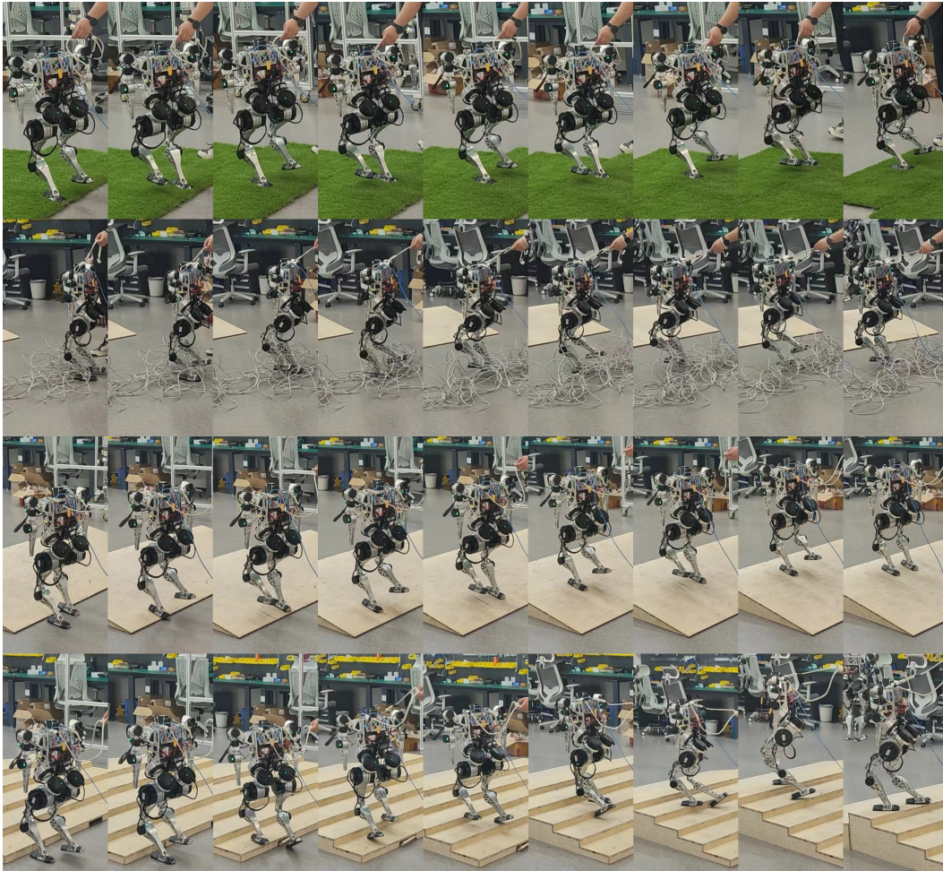
Figure 9: The sequence of images presented illustrates the diverse terrains our robot navigates with proficiency, ranging from the soft contours of grasslands to the challenging unevenness of wire-strewn areas, the inclines of varying gradients, and the ascents and descents of stairs. Each scenario, captured in a vertical progression from top to bottom, demonstrates not only the robot's adaptability but also its ability to maintain equilibrium on surfaces that demand different levels of traction and stability.
